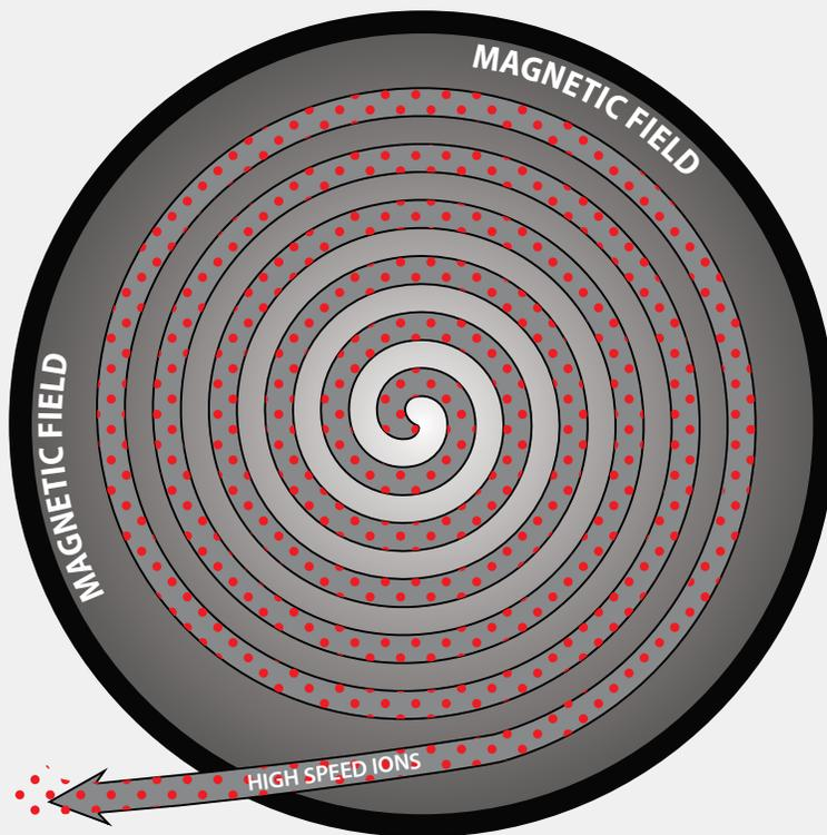
**Cyclotron Particle Accelerator**
